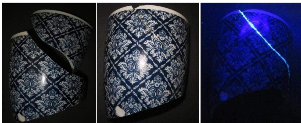
Figure 1. Picture depicting the bonding of a broken specimen design (left) by the adhesive and the visibility of the broken joint under normal light (middle) and long-wavelength UV light (right)
